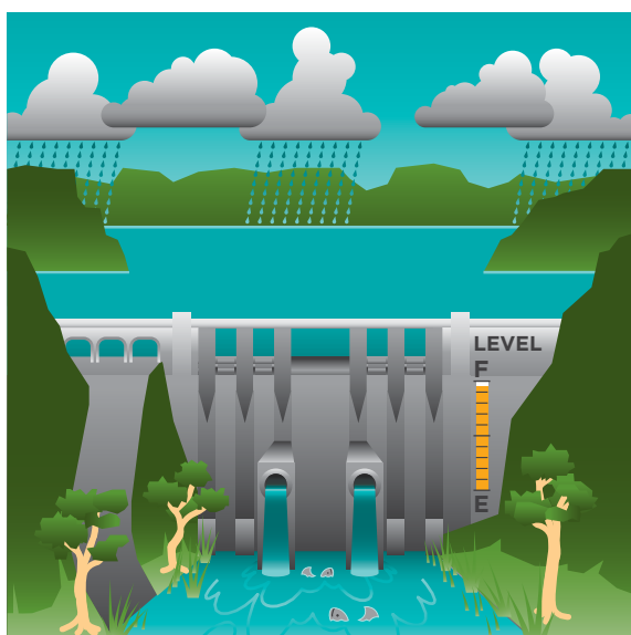
FIGURE 9A: High dam storage levels, high rainfall - high environmental flow release
